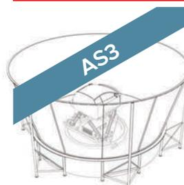
The ultimate complete vehicle simulator offering the highest possible level of immersion thanks to its high contrast and high resolution visual system with additional 360-degree yaw motion. Extra stiff dynamic platform, suitable for multiple applications such as vehicle dynamics, ADAS and HMI testing.
